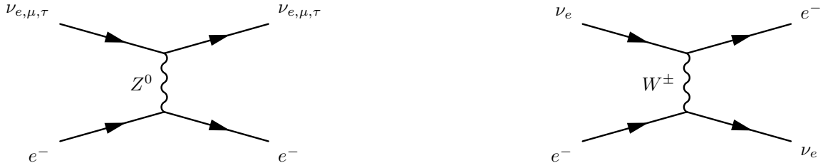
Figure 2.5: First-order Feynman diagrams for neutrino-electron elastic scattering. All neutrinos may scatter on electrons via a neutral-current interaction involving the exchange of a virtual Z^0 (left). Only electron neutrinos may scatter on electrons by the mediation of a charged virtual W particle (right).
